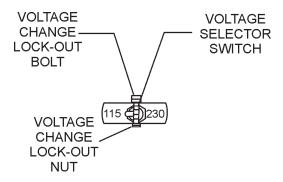
Figure 6. Voltage Change Switch
